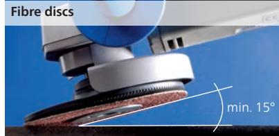
Using COMBICLICK helps to avoid scratches caused by protruding clamping pieces, and exploits the abrasive material that is available.
