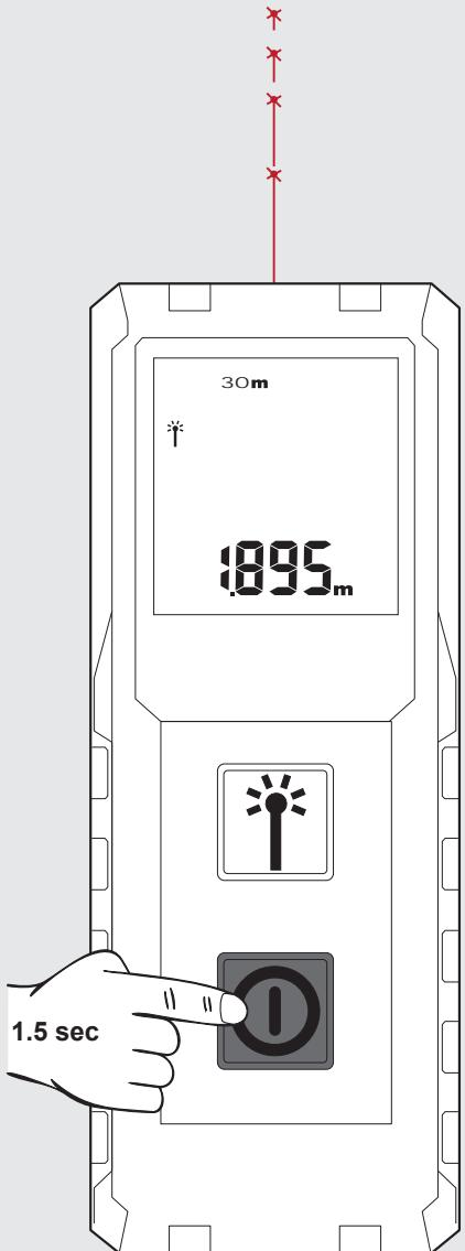
To freeze the measurement, press the measure button.
