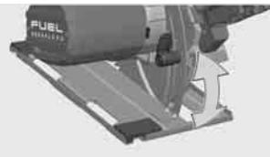
Adjust the cutting depth to the thickness of the workpiece. Less than a full tooth of the blade teeth should be visible below the workpiece.
