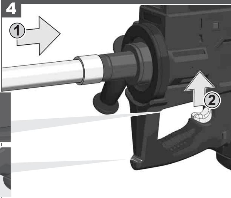
When the green indicator light turns on and/or the work light flashes, insert into the tubing and release the trigger.
