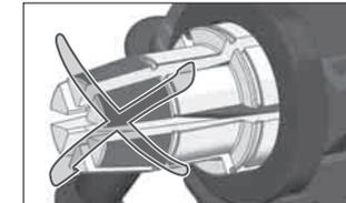
Rotate the six expander segments in the clockwise direction. The head will rotate freely. The head should not rotate counterclockwise.
