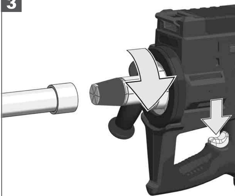
Pull and hold the trigger to initiate the rotation of the expander head. Do not insert into the tubing!
