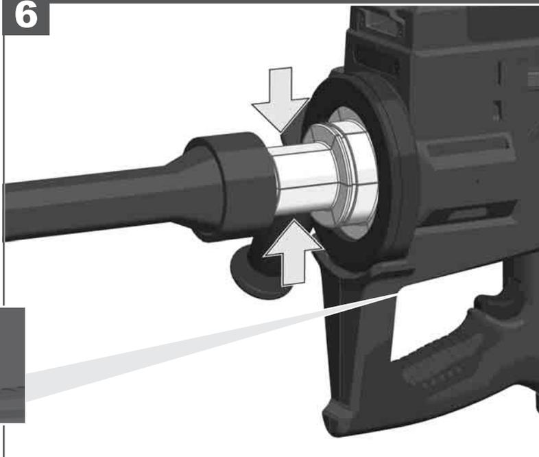
When the expander reaches maximum diameter it will automatically retract and the green LED blinks 3 times.
