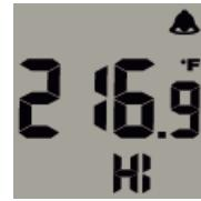
2. Press the up or down arrow soft keys to toggle between temperatures. Wait 5 seconds for the ranges to save and exit.
