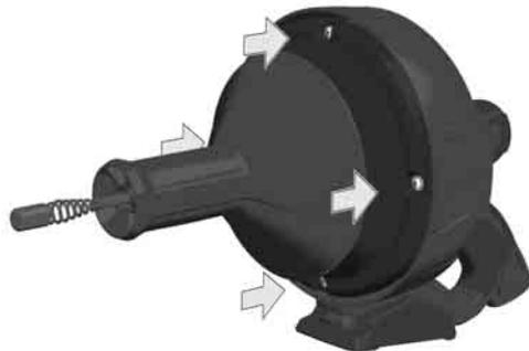
Wrap the cable carefully into the container.
